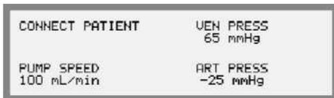
The connect patient overview menu, which gives current information on the most important parameters during patient connection, will be shown on the Information Display. To monitor the patient's blood access before blood has been detected in the venous blood line; read off current arterial pressure below ART PRESS and current venous pressure below VEN PRESS. The blood flow rate is displayed as PUMP SPEED until blood is detected in the venous blood line.
