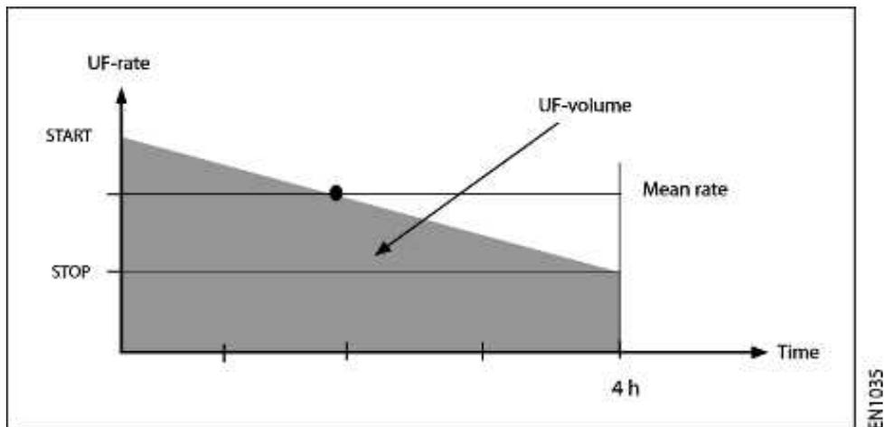
Figure 7:2 Decreasing linear graph for UF rate profiling
