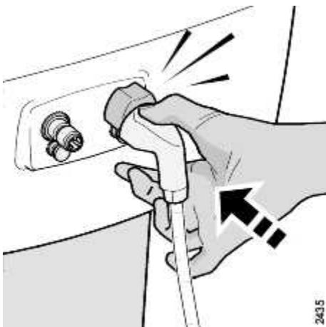
Release the button and simultaneously **push the connector into place until it clicks in**. The small button positioned just below the safety coupling will now be depressed which means that the connector is correctly attached to the machine.
