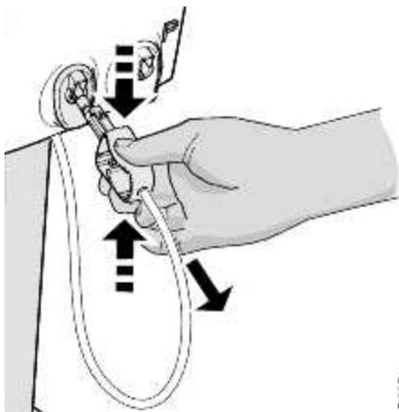
**To remove** the connector from the port; **compress the connector** as shown in the corresponding figure, **before pulling the connector out.**
