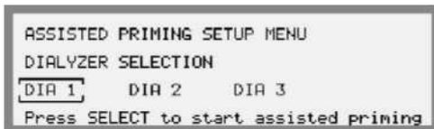
2. Select alternative in the ASSISTED PRIMING SETUP MENU using the *Keypad*.
