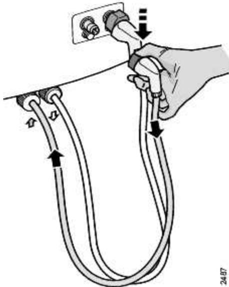
4. Disconnect the inlet dialysis fluid tube from the safety coupling of the machine; remove it in the same way as the outlet dialysis fluid tube described in the former point 1 in these instructions. The spent dialysis fluid flows **to the machine from the dialyzer** via this tube. A small arrow, fixed just below where the tube comes out from the machine, shows the flow direction.
