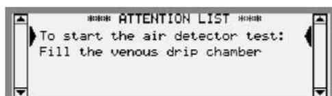
4. Fill up the level in the venous drip chamber (while the blood pump is running) using the level adjustment knob (anticlockwise direction). Adjust the level so it is well above the air detector head. Note that if the venous drip chamber is not being filled at the beginning of the priming procedure, an attention alarm without buzzer will appear to request the operator to do so.
