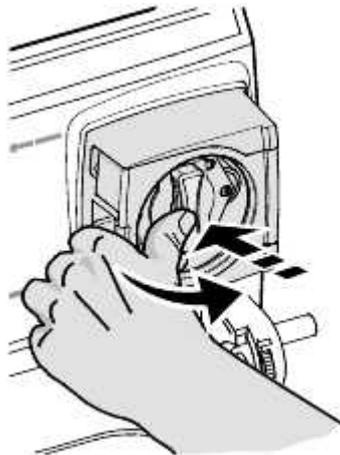
3. Open the cover of the blood pump and turn the blood pump manually.
