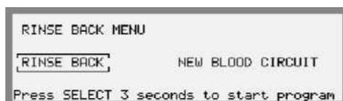
2. When RINSE BACK has been selected, press the *Select key* for 3 seconds to activate discontinuing mode. The menu will change and request the operator to press the flashing *Blood pump button* when ready for rinse-back.
