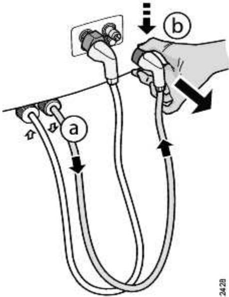
**To remove** the dialysis fluid tube from the safety coupling; **press and hold the button on the dialysis fluid tube** as shown in the corresponding figure (**(b)**), before removing it from the safety coupling.
