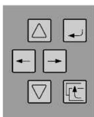
The *Keypad* consists of *Cursor keys*, *Display Up/Down keys*, *Select key* and *Back key*.
