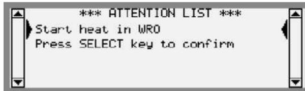
Follow the attention alarm request according to the instructions in the Operator's manual for WRO 300 H. Then press the *Select key* to confirm this.
