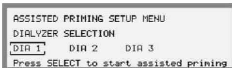
This menu will be displayed on the Information Display when assisted priming is active. If START BLOOD PUMP WHENREADY FOR PRIMING is displayed, briefly press the lit *Priming button* and select ASSISTED PRIMING using the *Keypad*. Then press the *Select key* for three seconds to activate assisted priming mode.
