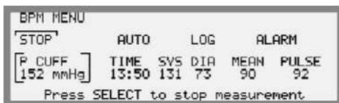
If the measuring process needs to be interrupted, when the BPM MENU is open, press the *Select key* to stop the procedure.
