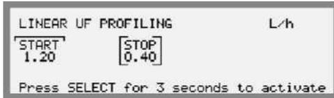
7. If linear graph (LINEAR) has been selected, set the start (START) value for UF rate. The stop value (STOP) will be automatically adjusted in proportion to the start value. This is to maintain the previously set UF volume for the following treatment.
