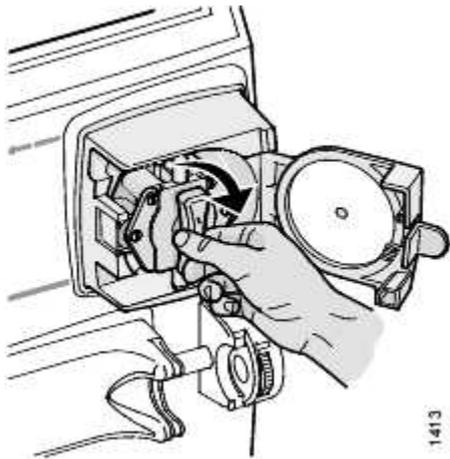
**To remove the blood pump rotor;** hold the handle and pull out. Then turn clockwise until the blood pump rotor loosens from the pump shaft.
