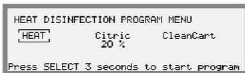
5. Start the program by pressing the *Select key* for 3 seconds until the *Rinse/Disinfection button* lights up.
