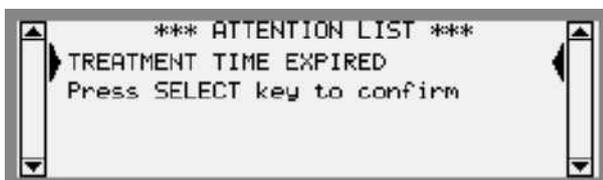
At this moment the UF rate will be automatically reduced to minimum UF rate as the set UF volume is achieved; the *UF Start/Stop button* will be extinguished to indicate this. The TMP alarm limits will automatically be widened. The time shown on the Time Display will continue to count down but will show negative figures.
