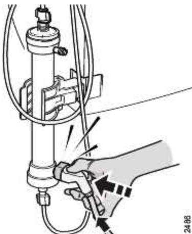
3. Release the button and simultaneously push the connector into place until it clicks in. Make sure that it clicks in properly to prevent leakage during treatment.
