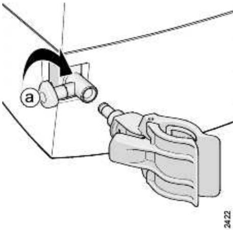
**Attach the Dialyzer Holder** to the holder arm and lock it into position using the locking screw (marked **a** in the corresponding figure) on the holder arm.
