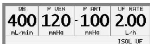
Activated isolated UF is displayed at the activity field of the Treatment Overview Menu on the Information display. During the phase, the accumulated values for ultrafiltration ACC UF and time ACC TIME will be displayed on the isolated UF menu. Press the *Fluid Path button*, select UF and then ISOL UF to view the menu.
