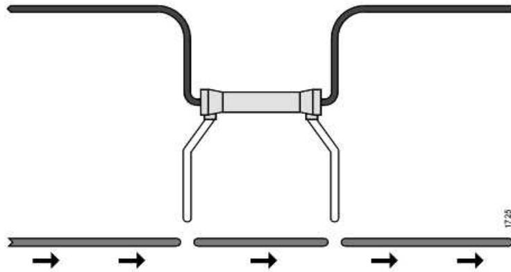
The bypass path lights green when the dialysis fluid preparation is ready (the conductivity level of the dialysis fluid is correct) for treatment. When the dialysis fluid is not correct the path is orange. The machine will automatically bypass the dialyzer during certain alarm conditions and during self-calibration.
