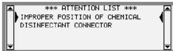
Note especially that the disinfectant connector must remain in the disinfectant container/disinfectant port and not be moved to the parking port before the program is complete. This is due that the chemical disinfectant is pushed back to the disinfectant container to empty the connector/intake tube at the end of the program.
