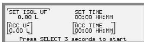
3. Set the ultrafiltration volume, SET ISOL UF, for the isolated UF phase.
