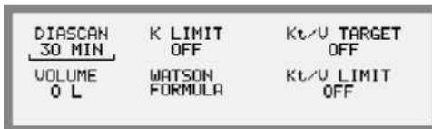
Activate the Diascan function by selecting SINGLE, 15 MIN, 30 MIN or 60 MIN. Deactivate the function by selecting OFF.
