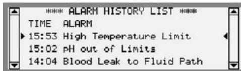
The time for when the alarm was generated is shown to the left on the Information Display.
