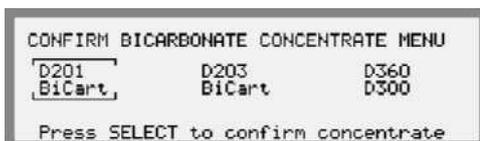
Note that at any time after confirming the concentrates, it is possible to enter the concentrate menus to check/select concentrates. Press the *Fluid path button* and select CONC. Go into the sub menus and check/select the connected concentrates using the *Keypad*.
