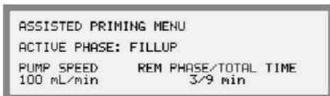
The procedure starts with the fill up phase. ACTIVE PHASE: FILLUP will be displayed.
