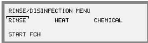
7. Start the rinse/drain program by pressing the *Rinse/Disinfection button* and select RINSE (the button lights up).
