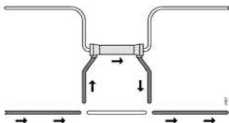
The dialysis fluid will now enter the dialyzer when the dialyzer path on the Flow Diagram lights up green. Especially note that the dialyzer should be filled from bottom to top to ensure proper de-airation.
