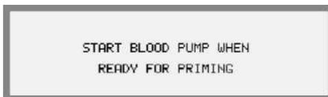
This menu will be displayed on the Information Display when manual priming is active. If the ASSISTED PRIMING SETUP MENU is displayed, briefly press the lit *Priming button* and select PRIMING using the *Keypad*. Then press the *Select key* for three seconds to activate manual priming mode.
