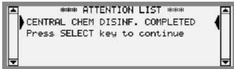
6. When the dwell time
