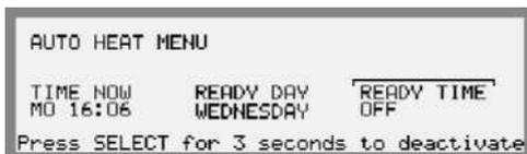
The *Select key* is used to activate and deactivate the auto heat function.
