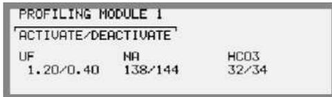
5. Check that the preset values in the model is correct. Activate the profiling model, by pressing the *Select key* for 3 seconds. Or, if desired, it is possible to activate the profiling function at any time during priming or treatment. Bear in mind, that the parameter settings of the complete model will be activated simultaneously. If necessary, it is possible to adjust the preset values of the parameters, refer to "Profiling without Preset Model", page 7:7.
