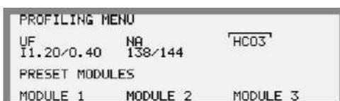
5. Press the *Select key* to go into the sub menu for HCO3 and the HCO3 PROFILING MENU will be displayed.
