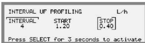
7. If step or interval graph (INTERVAL or (STEP) has been selected, first set the number of intervals/steps at the first position, then continue with the start (START) value for UF rate. The stop value (STOP) value for UF rate will be automatically adjusted in proportion to the start value. This is to maintain the previously set UF volume for the following treatment.
