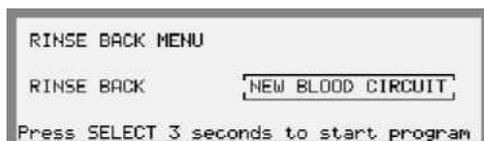
2. When NEW BLOOD CIRCUIT has been selected, press the *Select key* for 3 seconds to activate discontinuing mode.
