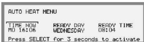
If changes are to be made or the auto heat process shall be inactivated, enter the AUTO HEAT MENU as described above.
