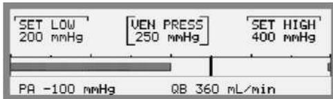
5. If desired, adjust the automatically set venous pressure alarm limits as necessary using the *Keypad*. Start by adjusting the high alarm limit. Then, during the arterial phase, gradually adjust the low venous pressure alarm limit as well. Make sure that the venous pressure alarm limits remain within the limits recommended by the clinic for that particular patient's blood access. See the next following Note for further information about this setting.
