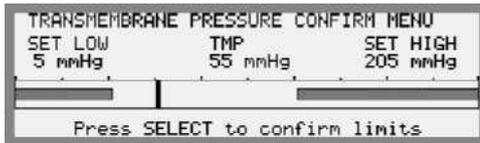
6. When the TRANSMEMBRANE PRESSURE CONFIRM MENU is displayed on the Information Display, press the *Select key* to confirm the settings i.e. that the current TMP value and the automatically set TMP alarm limits are set in accordance with the current UF rate and the UF coefficient of the dialyzer being used.
