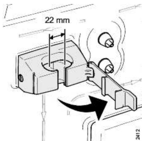
The air detector head is designed for a drip chamber with a diameter of 22 mm. Instructions on how to attach the venous drip chamber of the venous blood line in the air detector, can be read in "Venous Blood Line - Attach" on page 4:28 in part 1.
