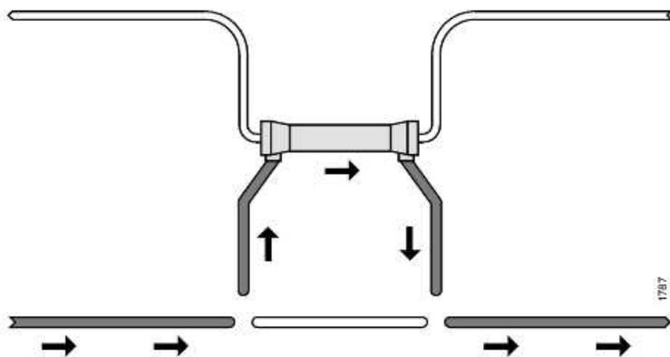
If the dialysis fluid tubes are connected to the safety couplings, the fluid will circulate within the machine. If they are connected to the dialyzer, the fluid will enter the dialyzer at that time. See "Dialysis Fluid Tubes - Attach" starting on page 4:35 in part 1 for instructions on how to properly attach the dialysis fluid tubes to the dialyzer.
