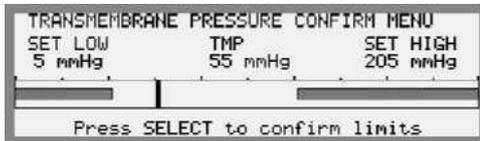
7. When the TRANSMEMBRANE PRESSURE CONFIRM MENU is displayed on the Information Display, press the *Select key* to confirm the settings i.e. that the current TMP value and the automatically set TMP alarm limits are set in accordance with the current UF rate and the UF coefficient of the dialyzer being used.
