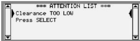
Check cause, adjust treatment parameters to increase clearance or adjust the alarm limit for clearance as above.
