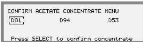
Note that at any time after confirming the concentrates, it is possible to enter the concentrate menus to check/select concentrates. Press the *Fluid path button* and select CONC. Go into the sub menus and check/select the connected concentrates using the *Keypad*.
