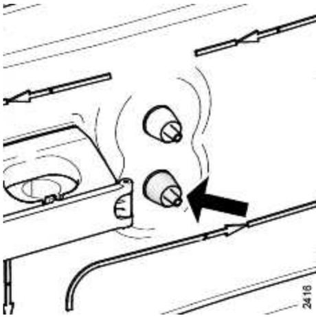
6. **Arterial Pressure Transducer Connector**
