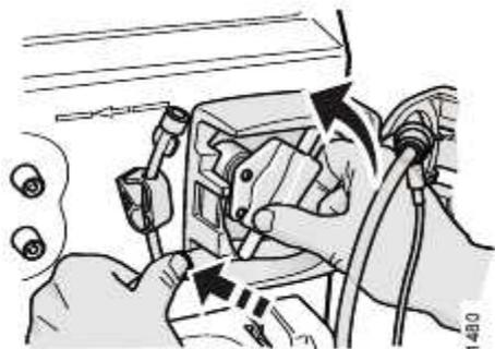
Press on the blood pump segment at the point shown in the figure before turning the blood pump rotor in an anti-clockwise direction. This is to hold the segment collar outside the pump housing while threading it.
