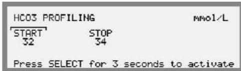
6. Set the start *START* and/or stop *STOP* values for bicarbonate.
