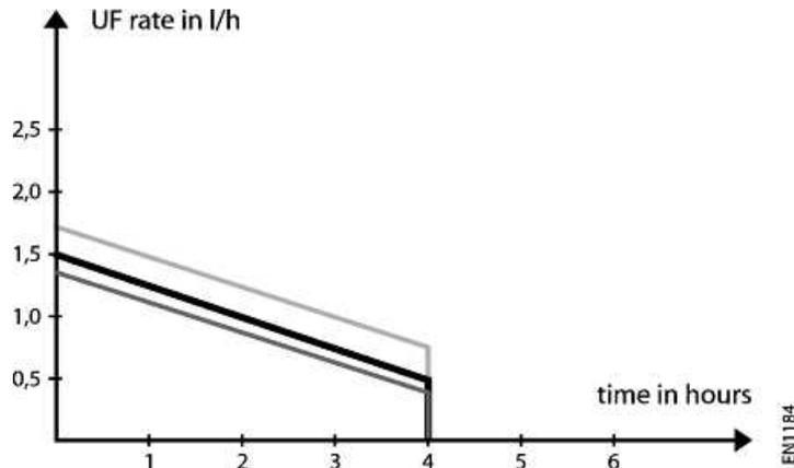
Figure 7:5 Change of UF rate linear graph when UF volume has been changed
