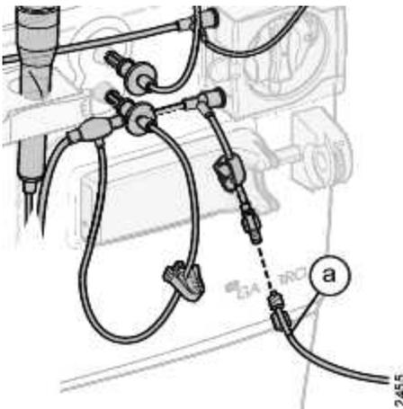
There is also the possibility of connecting the infusion line to the extracorporeal blood circuit pre-blood pump, **i.e. before the blood pump**. The corresponding figure shows pre-blood pump connection of infusion. The infusion line is marked **a**.
