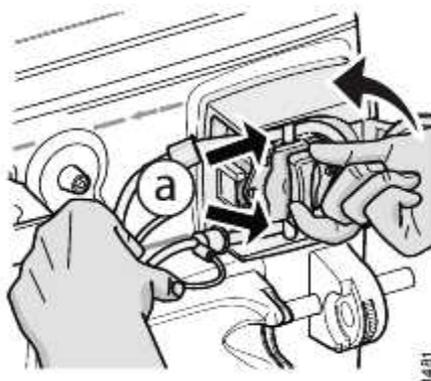
Continue turning the blood pump rotor in an anti-clockwise direction, while holding the segment, to thread the segment through the blood pump. The pins on the blood pump rotor, pointed out as **a** in the figure, hold the segment in place.
