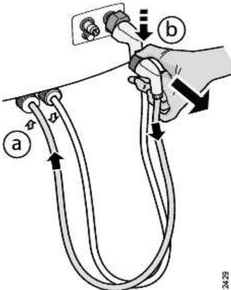
Remove the inlet dialysis fluid tube in the same way as the outlet dialysis fluid tube described in the previous point (2).
