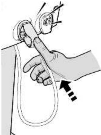
**To correctly attach** the connector to the port; insert the connector into the port and **push it into place until it clicks in.**
