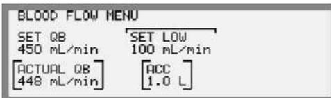
2. If desired, press the *Blood Path button* and open the BLOOD FLOW MENU using the *Keypad*. Check/adjust the low alarm limit for blood flow rate in SET LOW as necessary.
