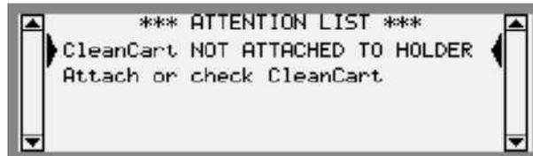
appears, open the latches of the BiCart holder and place the CleanCart cartridge to the holder in a similar way as when you place the BiCart cartridge to the holder. Default, the cartridge can be left in the holder during the entire program (up until next function check is started) and will automatically be emptied. The program will now start, continue to point 9 in these instructions.
