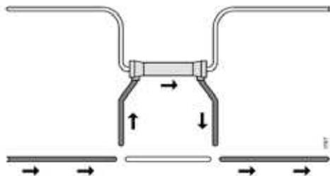
The dialysis fluid will now enter the dialyzer when the dialyzer path on the Flow Diagram lights up green. Especially note that the dialyzer should be filled from bottom to top to ensure proper de-airation.
