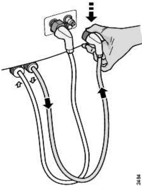
1. Disconnect the outlet dialysis fluid tube from the safety coupling of the machine; press and hold the button on the dialysis fluid tube before removing it from the safety coupling. The newly prepared, fresh dialysis fluid, flows **from the machine to the dialyzer** via this tube. A small arrow, fixed just below where the tube comes out from the machine, shows the flow direction.
