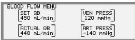
1. Check/adjust the blood flow rate (SET QB) to the required value suitable for the particular patient using the *Blood Pump Up/Down keys*.
