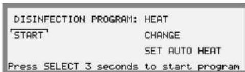
4. Check that HEAT is displayed as selected program. If HEAT is displayed, continue to point 4. If not, do point 4.a and 4.b before continuing to point 5.
