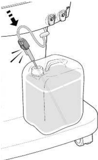
7. If the disinfectant connector is still connected to the parking port when the filling phase of the program starts, the following attention alarm will be generated:
