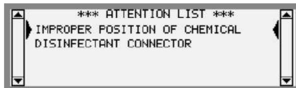
Note especially that the disinfectant connector must remain in the disinfectant container/disinfectant port and not be moved to the parking port before the chemical disinfectant program is complete. This is due that the chemical disinfectant is pushed back to the disinfectant container to empty the connector/intake tube at the end of the program.
