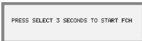
If a new treatment is to be started directly after the disinfection program, press the flashing *Priming button* briefly and PRESS SELECT 3 SECONDS TO START FCH will be displayed. Press the *Select key* for 3 seconds to start a new function check and simultaneously reset previous values to zero.
