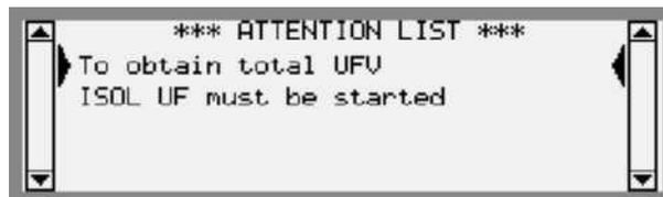
6. Check that the previously set values are the correct ones and activate isolated UF by pressing the *Select Key* for 3 seconds. Isolated UF will now be activated.
