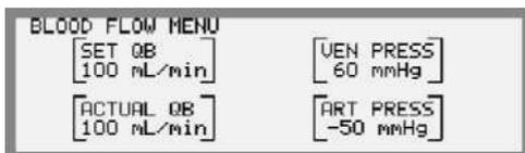
10. Set the required blood flow rate suitable for the patient using the *Blood Pump Up/Down keys*; the blood flow menu will be displayed, adjust SET QB. Especially note that the blood flow rate in SET QB and ACTUAL QB shown in the blood flow menu on the Information Display, is the blood flow rate when the blood pump is running in the arterial phase of the single needle cycle. It is **not** the mean blood flow rate for the single needle treatment.
