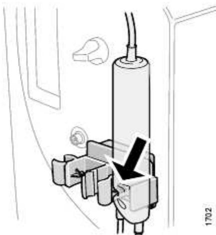
2. The edge inside the holder should fit into the groove of the expansion chamber as shown in the corresponding figure.
