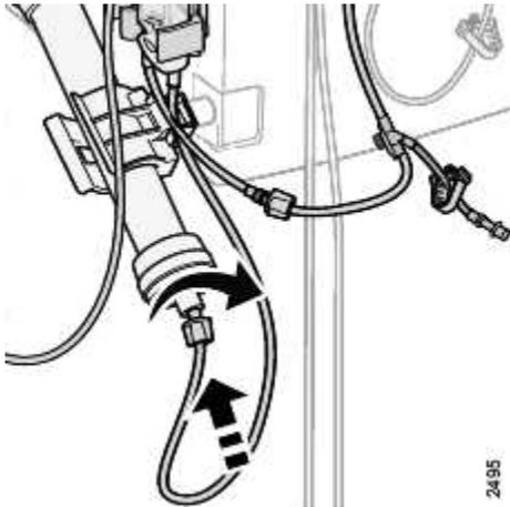
4. Connect the blood line with the expansion chamber to the dialyzer.
