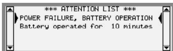
When only one minute remains of battery power an attention alarm will be displayed:
