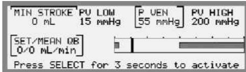
7. Activate the single needle function by pressing the *Select key* for 3 seconds. If desired adjust the alarm limit for minimum stroke volume MIN STROKE.
