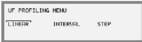
6. Select LINEAR , INTERVAL or STEP profiling using the *Select key*. and continue by following the corresponding instructions below.
