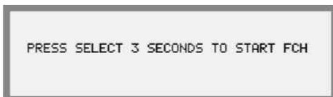
If a new treatment is to be started directly after the disinfection program, press the flashing *Priming button* briefly and **PRESS SELECT 3 SECONDS TO START FCH** will be displayed. Press the *Select key* for 3 seconds to start a new function check and simultaneously reset previous values to zero.
