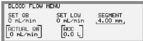
3. Press the *Select* key to open the parameter, adjust using the *Display Up/Down Keys*.
