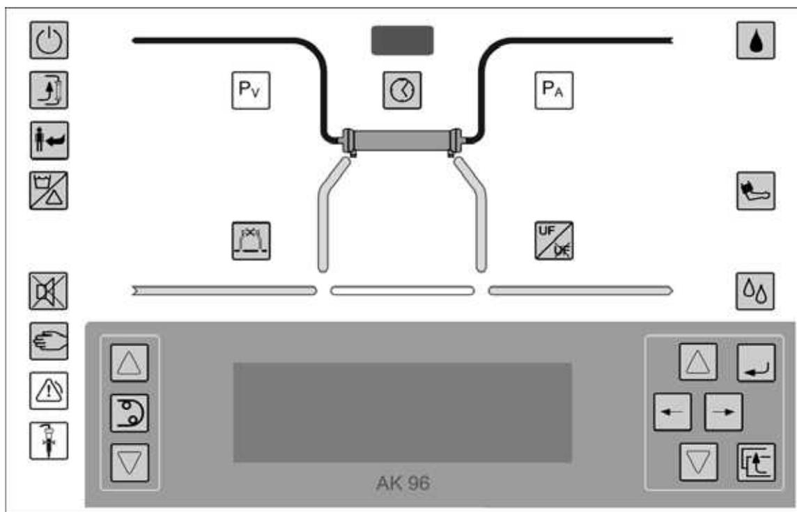
The Operator's Panel of the AK 96 dialysis machine consists of; a time display at the top of the panel, a Flow Diagram below this, function buttons, a key pad (setting keys) and an Information Display. The purpose of these components is to inform the operator of status and parameter values and also to guide the operator through the various procedures.
