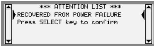
The operator must confirm the recovery after restart by pressing the *Select key*. The machine will then continue the treatment from where it was interrupted.
