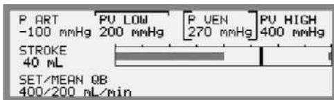
7. Check that the current stroke volume (STROKE) shows a proper value. See "Glossary of single needle parameters and key terms" on page 5:2 in part 1 for further information.
